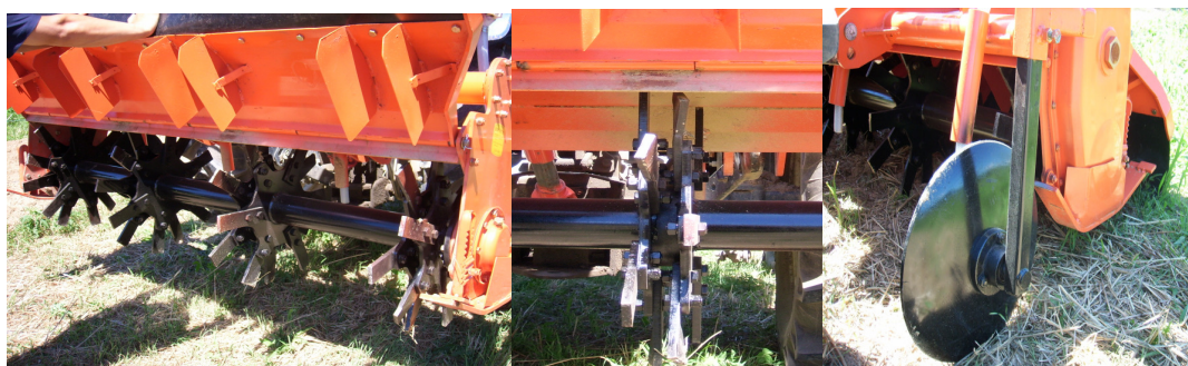
Figure 1. A four row tiller designed for reduce tillage.
