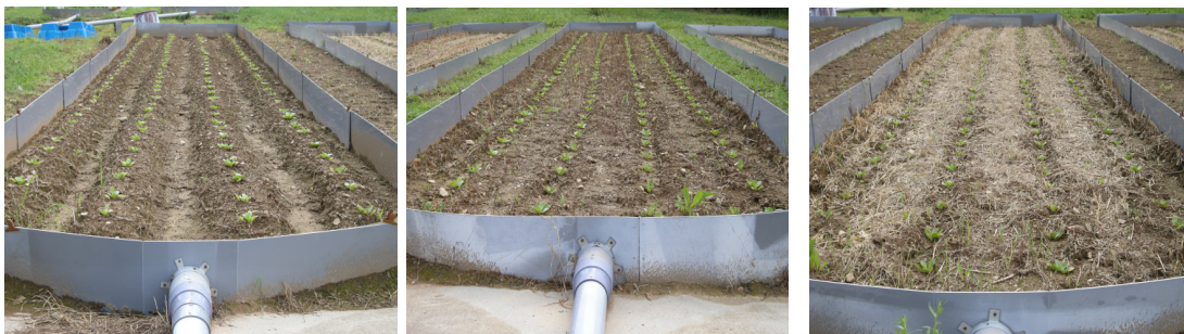
Figure 2. Lysimeter catchment to collect runoff and soil loss for conventional tillage (left), reduced tillage (center) and reduced tillage with rye mulching of Chinese cabbage.
